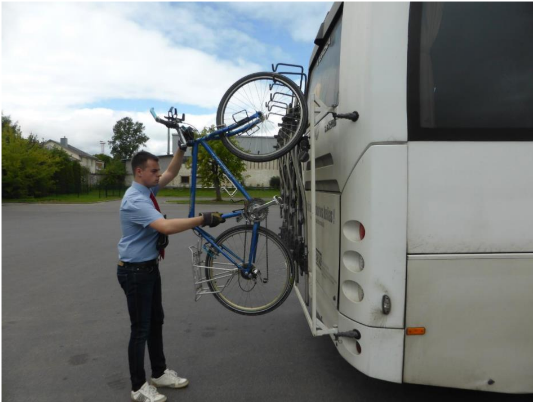
Intercity bus equipped with bicycle racks, Lithuania.
