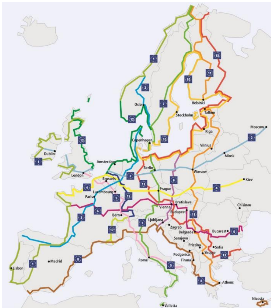
At the time of writing, there were 15 EuroVelo routes with a total length of over 70,000 km. North-South routes are identified by odd numbers, East-West routes and circuits by even numbers.
